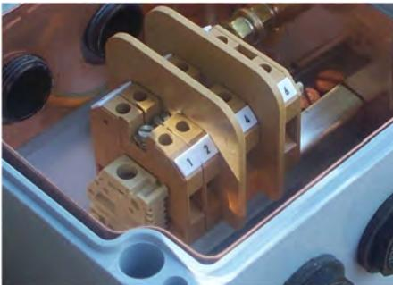
Each enclosure comes pre-drilled with four M20 tapped cable entries and is supplied with certified blanking plugs. The BPGA range of enclosures are ATEX and IECEx certified Ex'e' and are suitable for use in Category 2/Zone 1 & 21 and Category 3/Zone 2 & 22 areas according to EN 60079-14.
