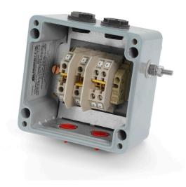
The BPGA range comprises three types of pre-assembled enclosure in two sizes. They are supplied complete with terminals, links, earthing and pre-drilled M20 threaded entries. BPGA enclosures are ideal for use as lighting, power and instrumentation junction boxes.
