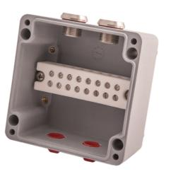
The BPGF is a fire resistant range comprising two enclosure sizes, pre-assembled with Abtech's ceramic terminal block. Supplied complete with four M20 threaded entries, two stainless steel plugs and two transit plugs.
