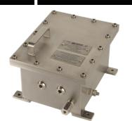
The SSD is an Ex d enclosure designed to house electrical and electronic apparatus within Zone 1 and 21 hazardous areas. Its Flameproof design allows potentially sparking equipment to be safely installed in areas where explosive gasses or dust may be present.
